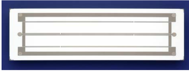
Fig. 1. Top view of the transient hot-bridge sensor layout. Each of the four tandem-strips is 100 mm in length and 2 mm in width.
